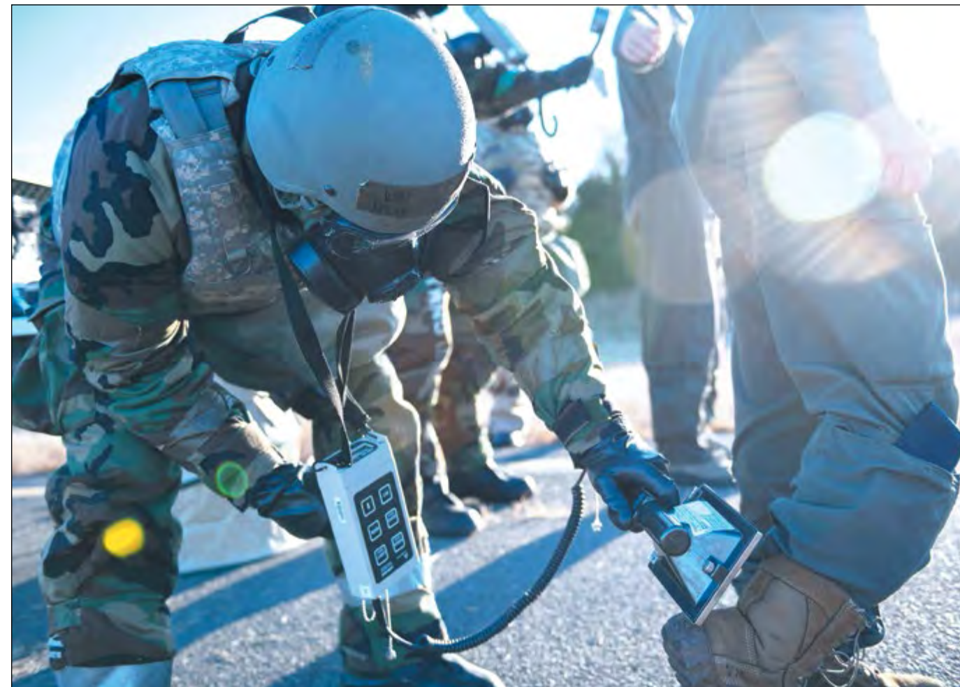
An Airman from the 19th Civil Engineer emergency management uses Alpha Probe-100 to monitor aircrew members for the presence of alpha radiation contamination as part of a simulated decontamination effort during phase II-B of ROCKI 20-01 Nov. 16 at Little Rock Air Force Base, Arkansas. Phase II-B marked the first time the radiological domain was tested as a portion of the exercise.
